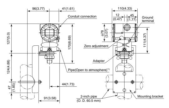
\*1: Applied to Model EJA530A with Measurement span code A, B, and C.
